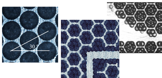
Fig. 14 Single shot screen, 100 l/cm, 30 ° and Masterscreen
