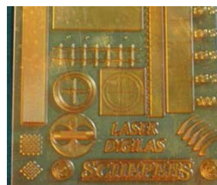
Fig. 6 Flexo polymer plate, ready for printing
