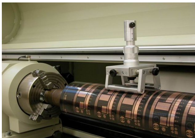
Fig. 10 Gravure cylinder after laser imaging of the mask with microscope
