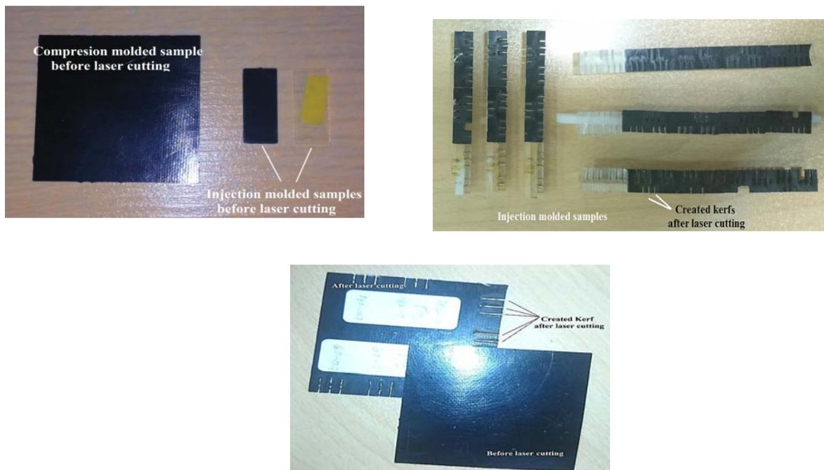
**Fig.1** the samples shape before and after laser cutting
