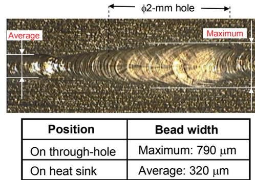
Fig. 6 Weld bead surface appearance near through-hole position.
