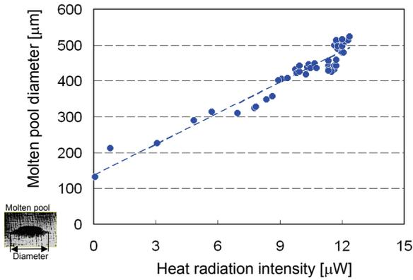
Fig. 4 Relationship between diameter of surface molten pool and intensity of heat radiation during spot welding at 75-W power.
