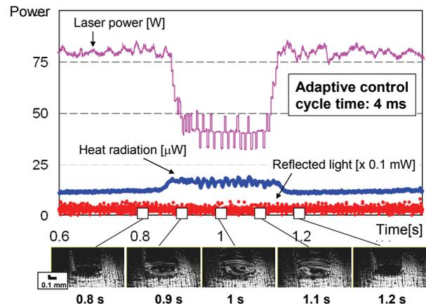
Fig.11 Monitoring results in micro bead-on-plate welding under adaptive control for suppression of bead expansion induced by surrounding conditions.
