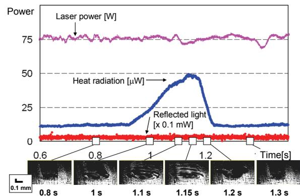
Fig. 8 Typical in-process monitoring results in micro bead-on-plate welding influenced by surrounding conditions of aluminum heat sink with φ2 mm through-hole.
