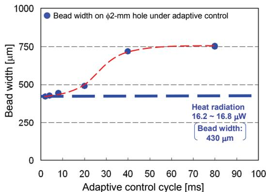
Fig. 13 Relationship between cycle of adaptive control and weld bead.
