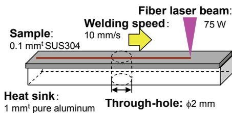
Fig. 5 Schematic illustration of micro bead-on-plate welding of 0.1-mm-thick stainless sheets with heat sink containing φ 2-mm through-hole by 75-W laser power.
