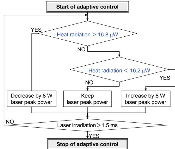
Fig. 10 Flow chart of adaptive control for stable production of weld bead width in micro bead-on-plate welding influenced by surrounding conditions.
