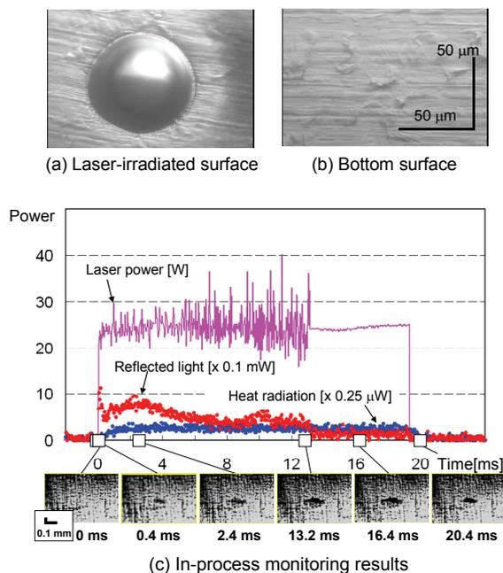
Fig. 2 Surface appearances and monitoring results of spot weld of SUS304 thin sheets, showing laser pulse shape, reflected light and heat radiation signals, and high-speed observation images of molten pool at 25-W laser power.
