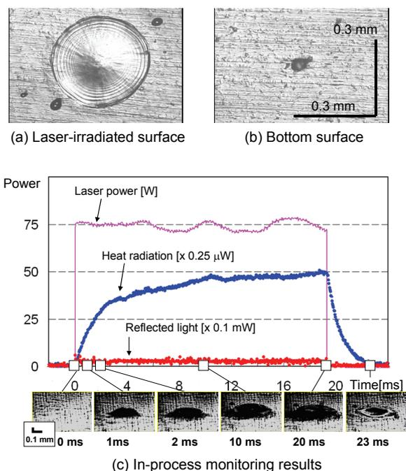
Fig. 3 Typical surface appearances and monitoring results in micro spot welding at 75-W laser power.
