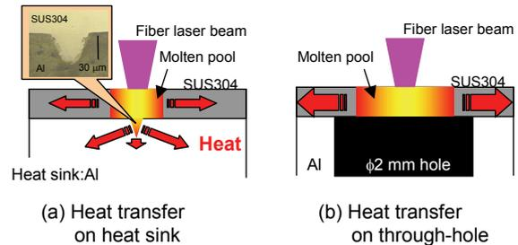
Fig. 7 Schematic illustration of heat transfer on heat sink and at through-hole position.
