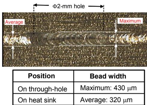
Fig. 12 Weld bead surface appearance near through-hole position under adaptive control with 2-ms cycle.
