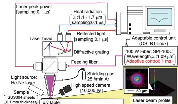
**Fig. 1** Schematic experimental set-up of in-process monitoring and adaptive control system with 100 W CW fiber laser.
