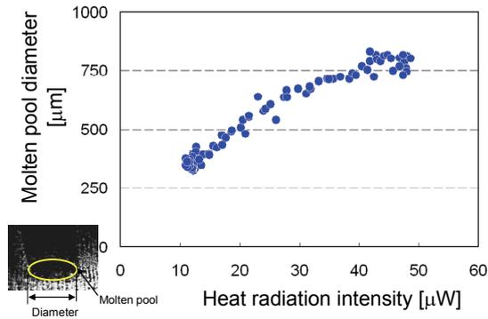
Fig. 9 Relationship between heat radiation and surface molten pool diameter perpendicular to welding direction.
