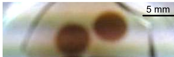
Fig 4 Colored areas formed by nanosecond UV laser pulses in the Ag-doped glass.
