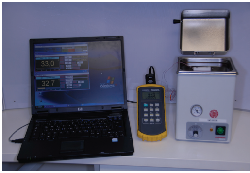
Fig. 2 Experimental setup for temperature recordings. The thermocouples attached to the implant surfaces were connected to the electronic measurement device and the temperature was directly read out to a personal computer.
