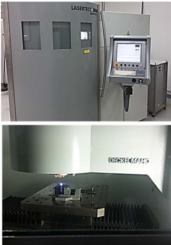
Fig. 1 Experimental setup of Nd:YAG laser beam micro-milling (LBMM)
