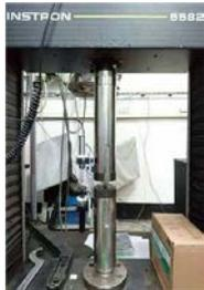
Fig. 3 Compression test setup of INSTRON 5582 system.
