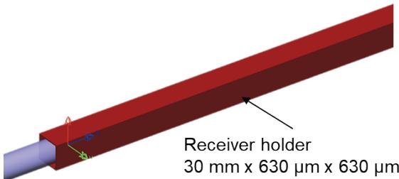
**Fig. 4** Model used in LightTools simulation. Processed fiber core (blue) and receiver surfaces (red).
