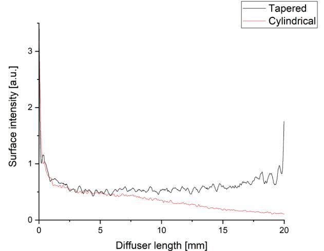
**Fig. 6** Radiation profile of tapered (black) and cylindrical (red) shaped diffuser measured with camera setup.
