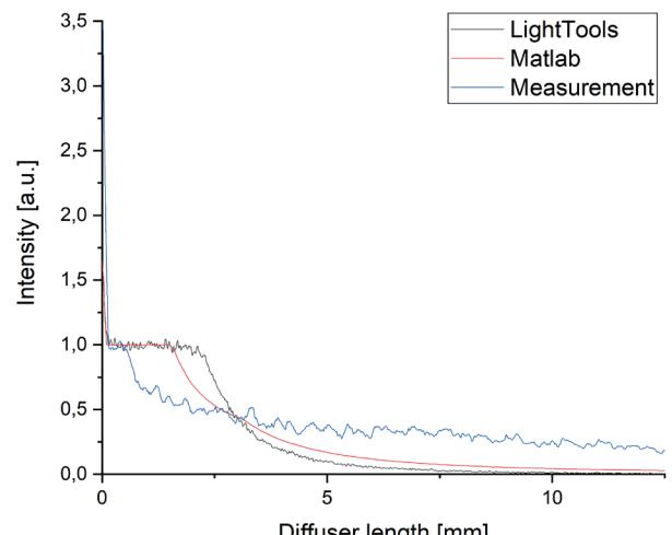
**Fig. 7** Radiation profile of tapered shaped diffuser simulated with Matlab (red) and LightTools (black).
