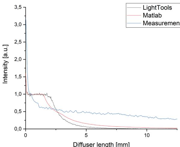
**Fig. 8** Radiation profile of cylindrically shaped diffuser simulated with Matlab (red) and LightTools (black).
