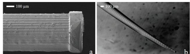
**Fig. 2** SEM images (JSM-7100F, JEOL, Tokyo, Japan) of manufactured fiber tips. - a: cylindrical, b: tapered.
