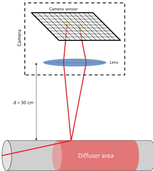
**Fig. 3** Schematic measurement setup to obtain the radiation profile of a fiber diffuser.
