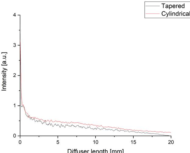
**Fig. 5** Brightness on the surface of a tapered (black) and cylindrical (red) diffuser measured with camera setup.
