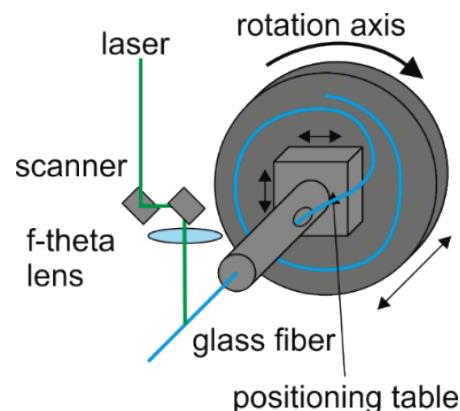
**Fig. 1** Schematic setup of ultrafast-laser fiber processig with rotational axis.
