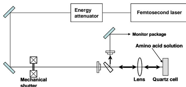
Fig. 1 Schematic diagram of the experimental arrangement.
