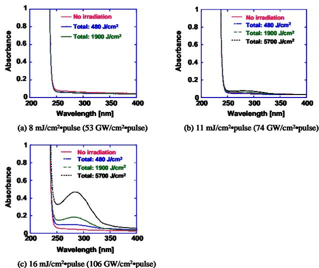
**Fig. 3** Ultraviolet absorption spectra of histidine for (a) 8 mJ/cm<sup>2</sup>•pulse (53 GW/cm<sup>2</sup>•pulse), (b) 11 mJ/cm<sup>2</sup>•pulse (74 GW/cm<sup>2</sup>•pulse), (c) 16 mJ/cm<sup>2</sup>•pulse (106 GW/cm<sup>2</sup>•pulse)
