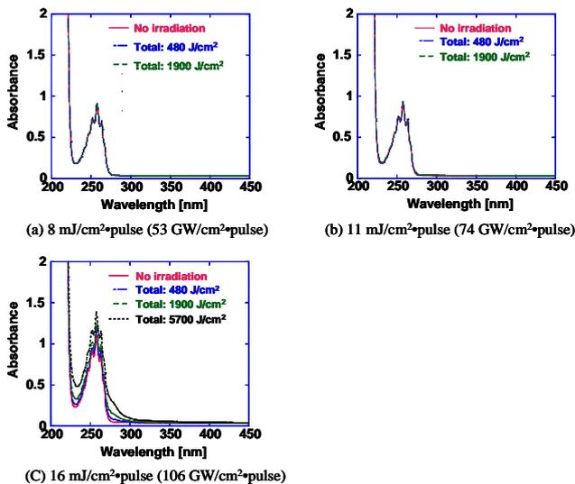
**Fig. 4** Ultraviolet absorption spectra of phenylalanine for (a) 8 mJ/cm<sup>2</sup>•pulse (53 GW/cm<sup>2</sup>•pulse), (b) 11 mJ/cm<sup>2</sup>•pulse (74 GW/cm<sup>2</sup>•pulse), (c) 16 mJ/cm<sup>2</sup>•pulse (106 GW/cm<sup>2</sup>•pulse)
