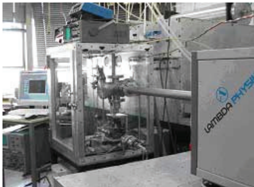
Fig. 1 157 nm micro-machining stage. The computer controlled CCD camera, the X-Y-Z- \Theta micro-translator, the focusing optics and the sample holder are indicated.
