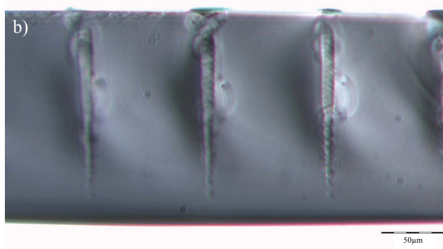
Fig 12 (a) Images of a 3D channel performed in the bulk of a PMMA at 515 nm and 7.5 nJ/pulse, (b) a cut has been made on the slide to observe the characteristics of the channels.
