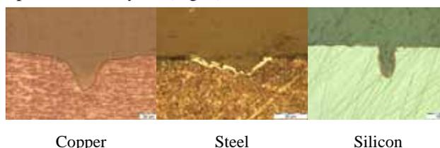
Fig. 8 Etched grinding patterns of different materials feed rate 0.5 mm/s, pulse energy 910 μJ
