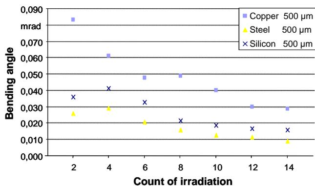
**Fig. 12** Bending angles reached with multiple irradiations
