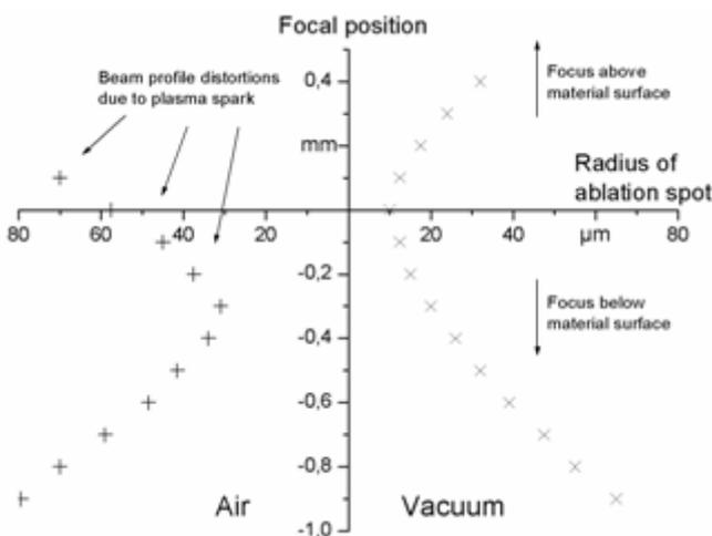
**Fig. 9** Beam profile of LIBRA CPA-System derived from measured ablation traces in air and vacuum
