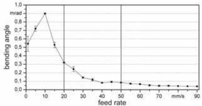
Fig. 3 Dependency of bending angle on laser feed rate
