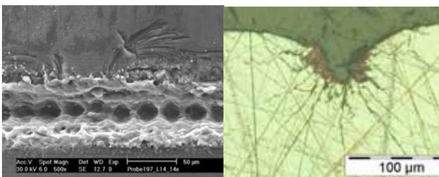
**Fig. 13** SEM-picture and etched grinding pattern of silicon after 14 processing steps, feed rate 25 mm/s, pulse energy 910 mW
