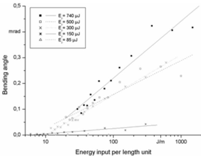
**Fig. 11** Bending angles achieved with different pulse energies
