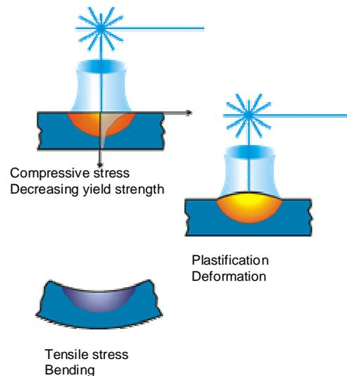
**Fig. 1** Temperature Gradient Mechanism
