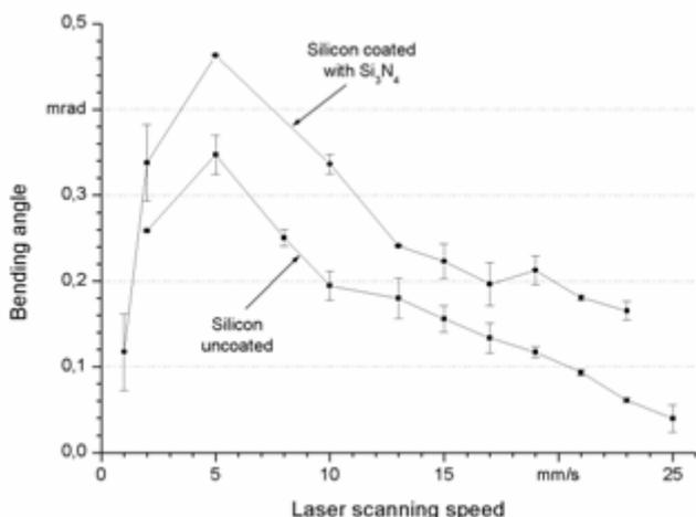
Fig. 6 Dependency of bending angle to feed rate for coated and uncoated silicon, laser Coherent LIBRA, 800 nm, 100 fs, 1 kHz, 750 μJ / pulse
