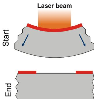
Fig. 2 Micro-adjustment by ultrashort pulse ablation of pre-stressed coating layers
