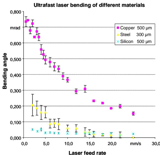
Fig. 7 Dependency of bending angle to laser feed rate for copper, steel and silicon, pulse energy 750 μJ
