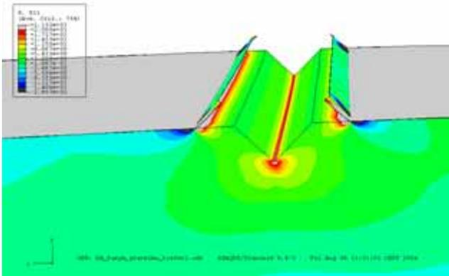
**Fig. 4** FEM-Simulation of a V-shaped, 50  $\mu\text{m}$  deep ablation trace and its effects on the stress distribution
