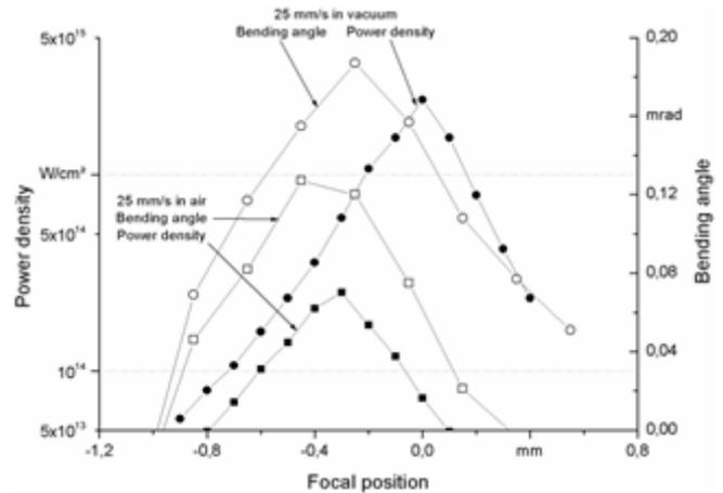
**Fig. 10** Bending angle and power density in air and vacuum
