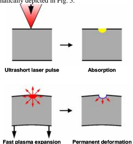
**Fig. 5** Micro-bending by ultrafast laser induced shockwaves – process model
