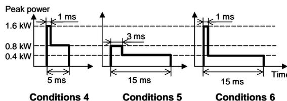
Fig. 10 Decrease welding conditions of laser peak power in pulsed YAG laser.
