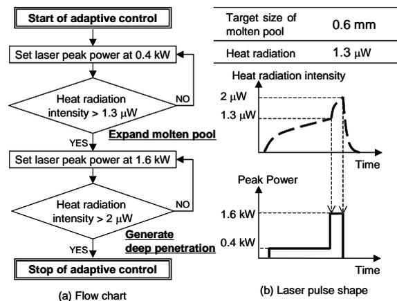
Fig. 14 Flow chart of adaptive control for reduction of spatters.
