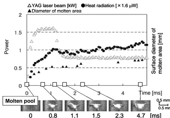
Fig. 11 Monitoring results of typical welding process caused by rapid decrease of laser peak power, showing laser pulse shape, reflected light and heat radiation signals, and high-speed observation images of molten pool.
