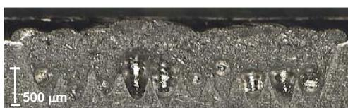
Fig. 17 Porosity in the cross section of weld bead under adaptive control for reduction of spattering.
