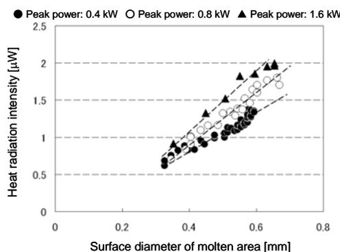
Fig. 5 Relationship between diameter of surface molten area and heat radiation at each laser peak power.
