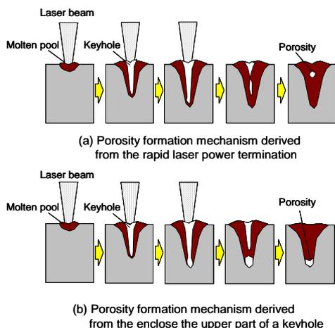
Fig. 18 Schematic drawing of porosity formation mechanism.
