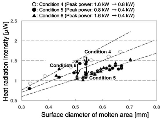
Fig. 12 Relationship between surface diameter of molten area and heat radiation with respect to laser power increase.
