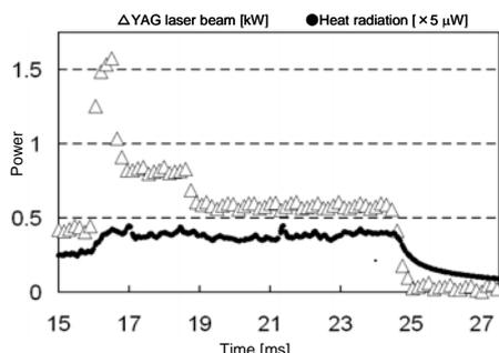
Fig. 21 Monitoring results of laser pulse shape and heat radiation signals under adaptive control for reduction of porosity.
