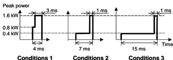
Fig. 7 Three welding conditions used, showing different laser peak power in pulsed YAG laser welding.
