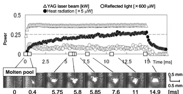
Fig. 3 Monitoring results of typical butt weld of pure titanium, showing laser pulse shape, reflected light and heat radiation signals, and high-speed observation images of spot weld molten pool.
