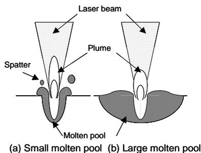
Fig. 13 Schematic drawing of easier generation of spatters from small molten pool but area.
