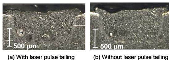
Fig. 20 Cross section of weld bead with or with laser pulse tailing in seam welding of 7/8 overlapped rate.
