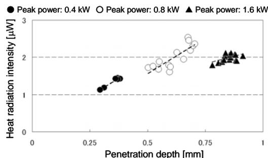
Fig. 6 Relationship between penetration depth and heat radiation at each laser peak power.
