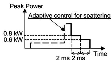
Fig. 19 Two-steps laser pulse tailing for prevention of porosity.
