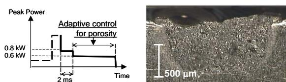
Fig. 22 Cross section of weld bead produced by laser with adaptively-controlled laser pulse tailing.
