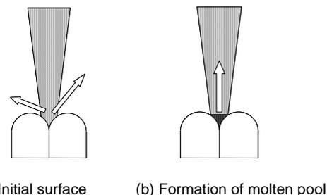
Fig. 4 Schematic drawing of laser beam reflection from titanium parts.
