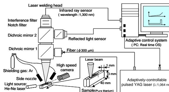
Fig. 1 Schematic experimental set-up of in-process monitoring and laser adaptive control system.
