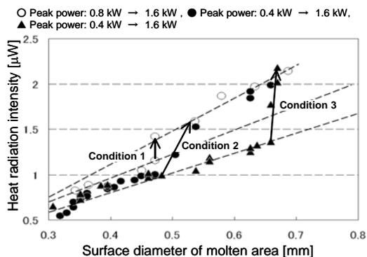
Fig. 9 Relationship between surface diameter of molten area and heat radiation with respect to laser power increase.
