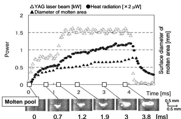
Fig. 8 Monitoring results of typical welding process caused by rapid increase of laser peak power, showing laser pulse shape, reflected light and heat radiation signals, and high-speed observation images of molten pool.
