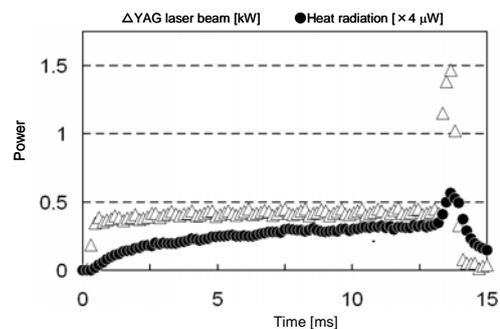
Fig. 15 Monitoring results of laser pulse shape and heat radiation signals under the adaptive control for reduction of spattering.
