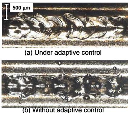
Fig. 16 Surface appearances of laser seam weld without adaptive control and under adaptive control for spattering reduction.
