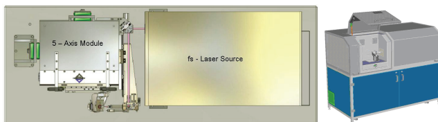
Figure 9: Left: Top view of 5-stage positioning module and laser head on granite base plate. Right: Housing with separate machining cabin and fume extraction
