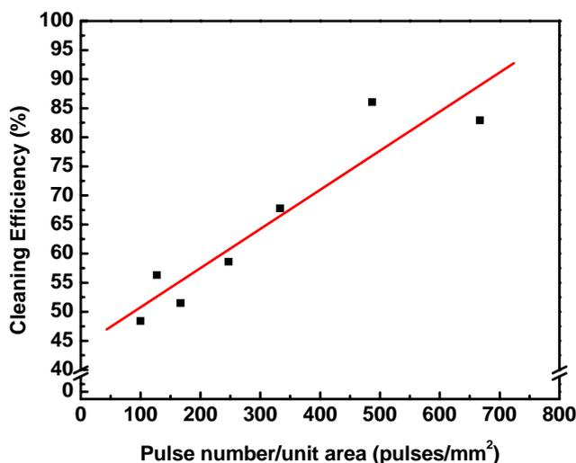
**Fig. 7** Cleaning efficiency of chilled laser cleaning under varying pulse number/unit area. Cleaning efficiency increases with pulse number/unit area. Standardized process parameters: laser fluence: 1.0 J/cm<sup>2</sup>, pulse repetition rate: 5 kHz, scan count: 1, scan count: 1, particles: 1 μm polystyrene (Duke Scientific 5100A), temperature: -2 °C.
