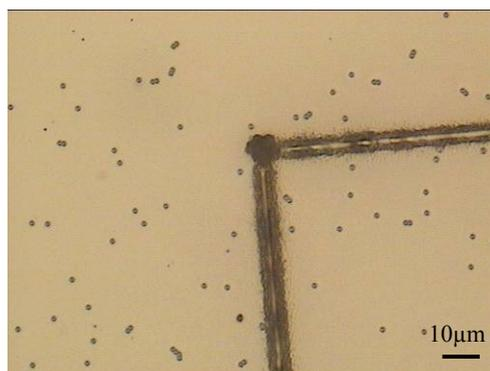
Fig. 4 Sample is marked by laser before laser cleaning to allow easy location of the same area for calculation of cleaning efficiency.
