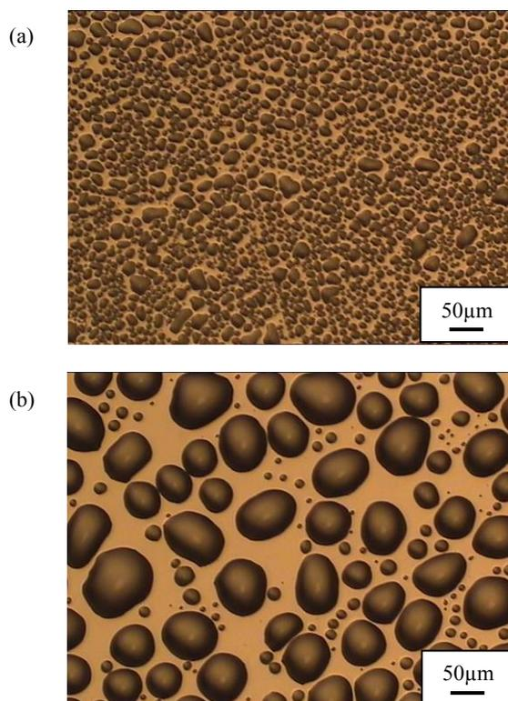
**Fig. 1** Optical microscope images of water film layer formed by (a) ambient water vapour condensation and (b) steam condensation.
