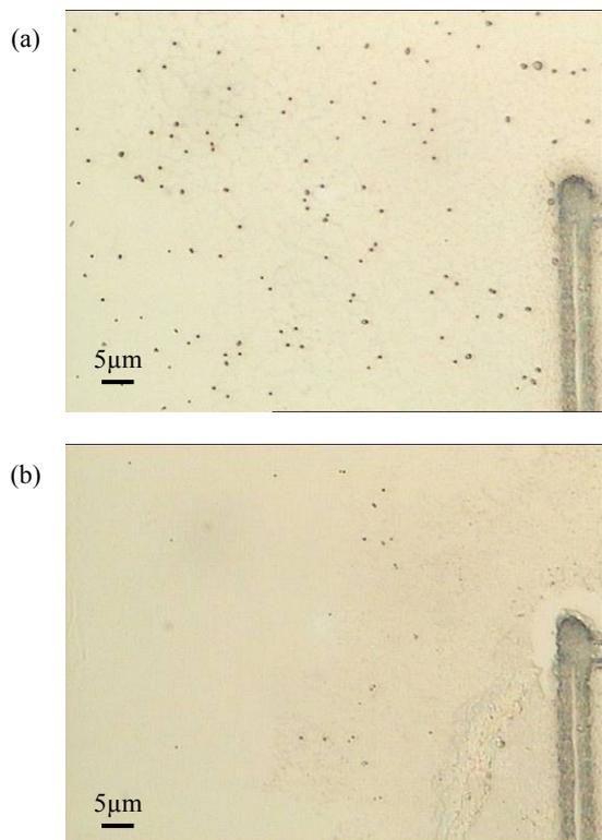
**Fig. 9** Optical microscope images before (a) and after (b) cleaning using CLC for 300 nm silica particles. Most of the silica particles are removed after the cleaning process. Process parameters: laser fluence: 1.0 J/cm<sup>2</sup>, pulse repetition rate: 5 kHz, pulse number/unit area: 208 pulses/mm<sup>2</sup>, scan count: 1, particles: 300 nm silica, temperature: -2 °C.
