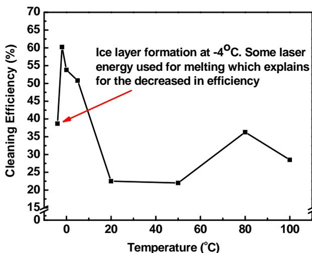
**Fig. 8** Cleaning efficiency of chilled laser cleaning under varying temperatures. Standardized process parameters: laser fluence: 1.0 J/cm<sup>2</sup>, pulse repetition rate: 5 kHz, pulse number/unit area: 133 pulses/mm<sup>2</sup>, scan count: 1, particles: 1 μm polystyrene (Duke Scientific 5100A).
