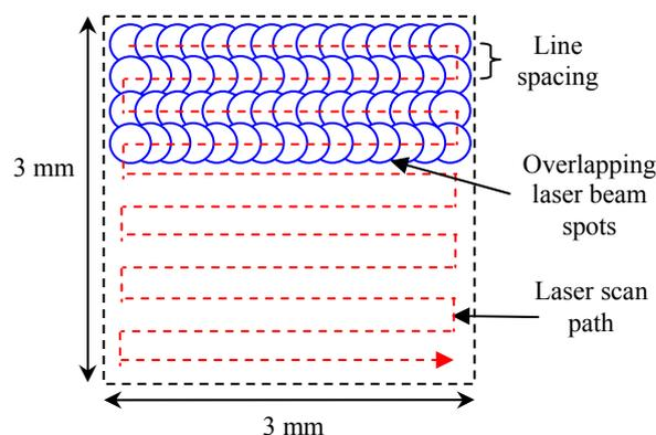
Fig. 3 Scan path taken by the laser during scanning on a 3 × 3 mm square area on the substrate surface.
