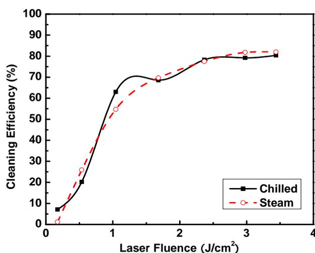
**Fig. 5** Cleaning efficiency of chilled and steam laser cleaning under varying laser fluence. Both techniques show comparable cleaning efficiencies at the same fluence and there is a general increasing trend of cleaning efficiency with laser fluence. Standardized process parameters: pulse repetition rate: 5 kHz, pulse number/unit area: 133 pulses/mm<sup>2</sup>, scan count: 1, particles: 1 μm polystyrene (Duke Scientific 5100A), temperature: -2 °C (for CLC).
