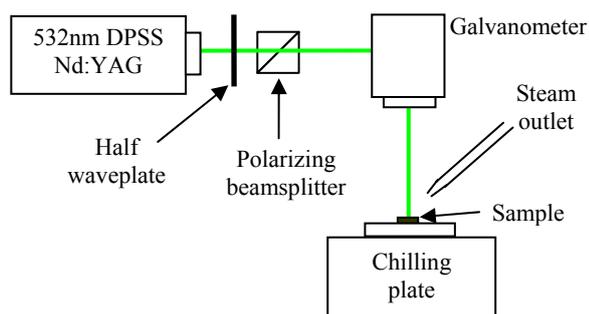
Fig. 2 Experimental setup for laser cleaning
