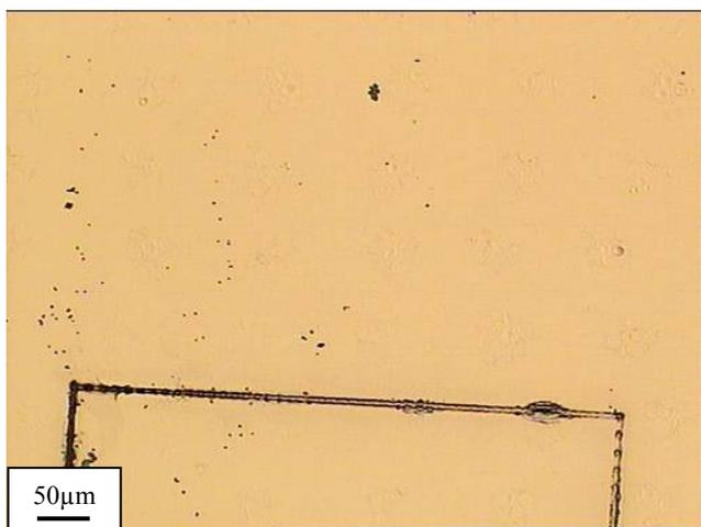
**Fig. 6** Optical microscope image of Si surface after the cleaning process shows melting at some areas. Process parameters: Laser fluence: 3.4 J/cm<sup>2</sup> pulse repetition rate: 5 kHz, pulse number/unit area: 133 pulses/mm<sup>2</sup>, scan count: 1, temperature: -2 °C (for CLC).
