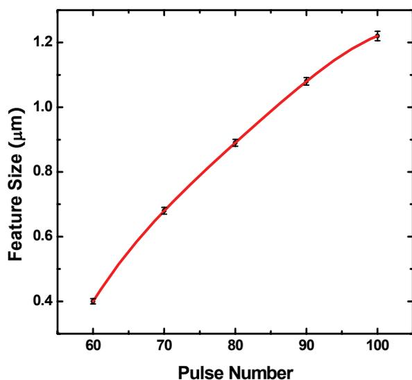
**Fig. 3** Dependence of feature size on a phase-change film on the number of pulses of femtosecond laser irradiation at a laser power of 200 mW.
