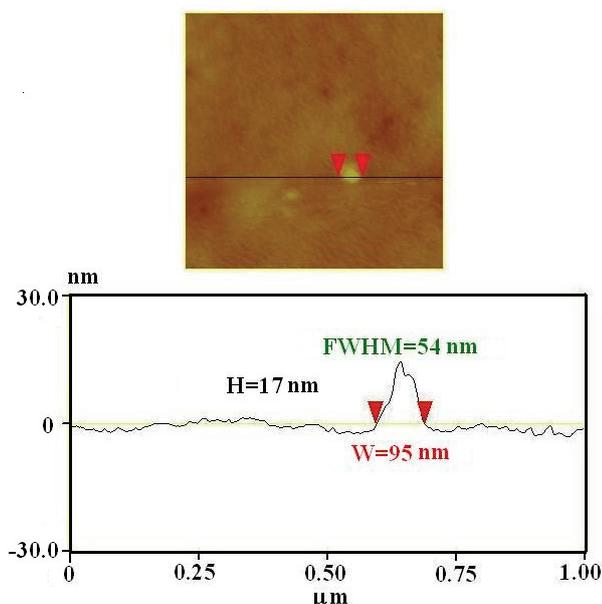
**Fig. 7** Line profile of a bump feature with a size of 95 nm and a full width at half maximum (FWHM) of 55 nm, and a height of 17 nm. It was fabricated at a laser power of 80 mW with 50 pulses of the laser irradiation with the GeSbTe film subsequently dipped into a 30% alkaline solution for 1 minute.
