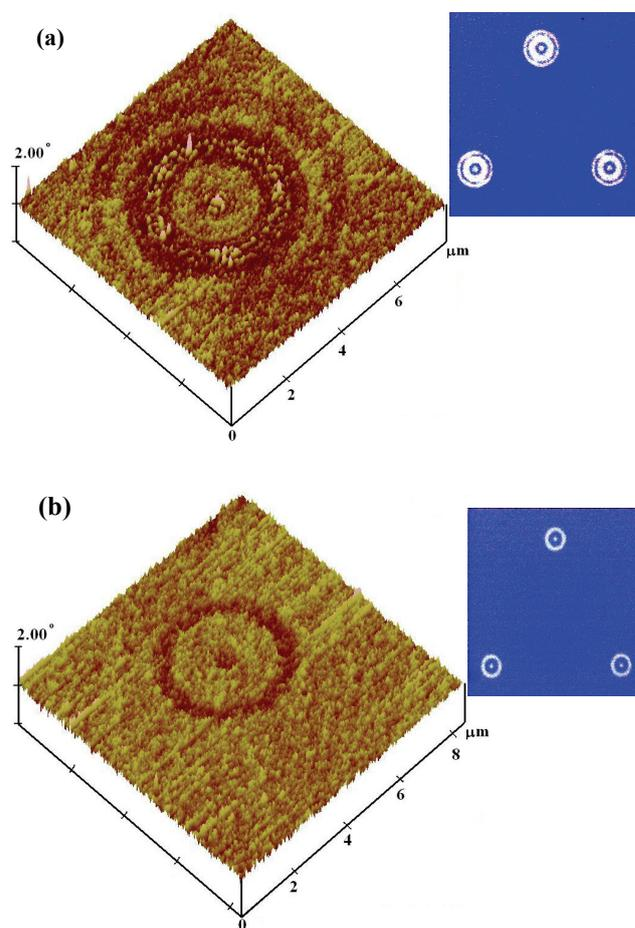
**Fig. 4** 3D EFM images of dot patterns on the phase-change thin films fabricated by the femtosecond laser irradiation through the MLA at an incident laser power of 140 mW and different MLA-to-sample distances.
