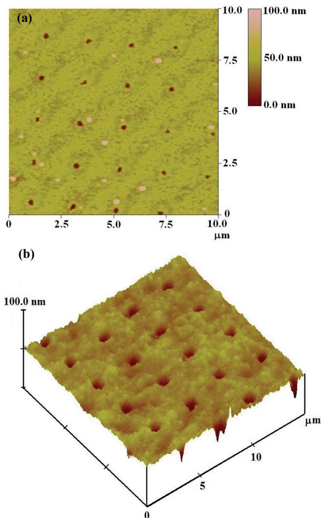
**Fig. 8** (a) 2D AFM image of SbTe film and (b) 3D AFM image of GeTe film patterned with a femtosecond laser at a laser power of 200 mW with 50 pulses and 100 pulses of the laser irradiation, respectively. The films were then etched by 30% alkaline solution for 30 seconds.
