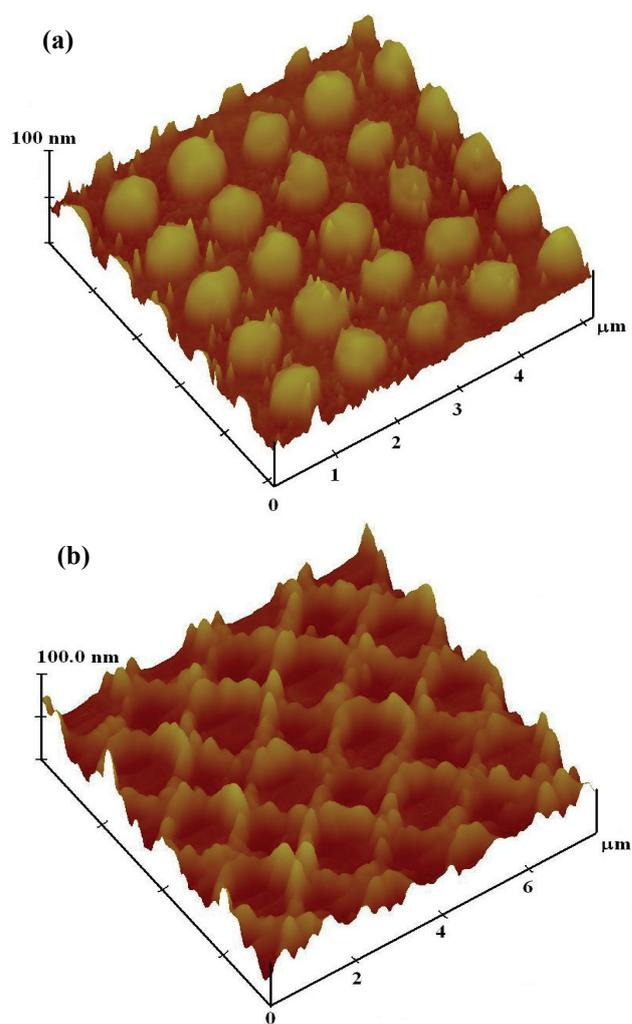
**Fig. 6** 3D AFM images of (a) pillar-arrays with a period of 1  $\mu\text{m}$  patterned with 70 pulses of the femtosecond laser irradiation by placing the GeSbTe film at the focal plane and (b) ring-wall features patterned with 90 pulses of the femtosecond laser irradiation by placing the film at the non-focal plane at a laser power of 200 mW.
