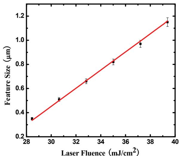
**Fig. 2** Dependence of feature size on the GeSbTe film incident laser fluence under 532 nm Nd:YAG laser irradiation through a MLA.
