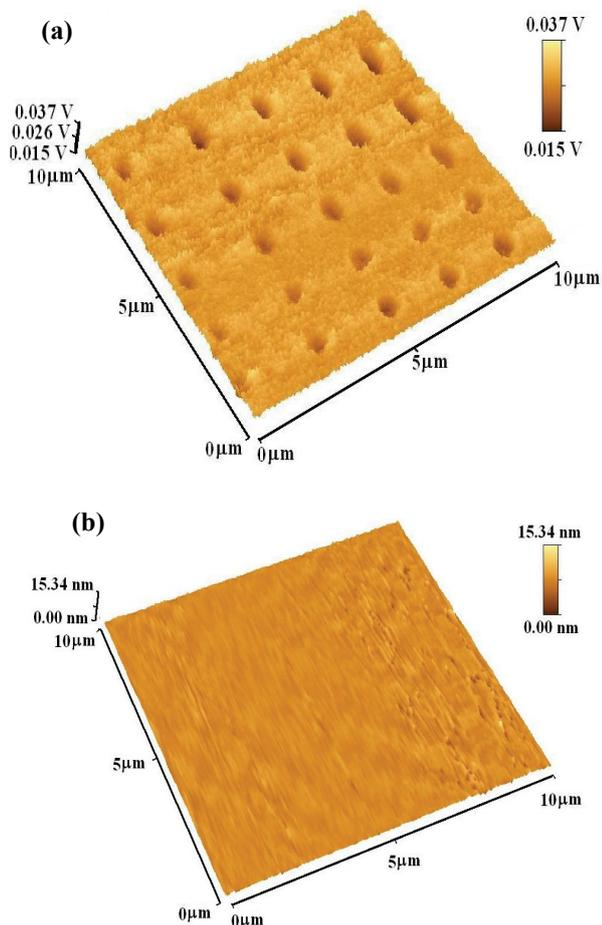
**Fig. 5** (a) 3D transmission NSOM image and (b) 3D topography image of crystalline dot features in the GeSbTe films produced by the femtosecond laser with 100 pulses irradiation through a MLA at a laser power of 200 mW.
