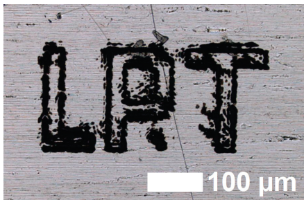
Fig. 2. Optical microscope image of a microstructure generated by SLM beam shaping. The sample material used was 1.4301 stainless steel.
