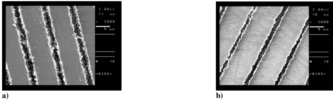
Fig. 7: a) SEM-image of a PMMA surface relief grating ( p = 0.3 \text{ mW} ) b) SEM-image of a fluorinated PMMA surface relief grating ( p = 0.3 \text{ mW} )
