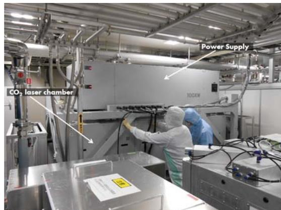
Fig. 21. Installation of new pre-amplifier in the “proto #2” CO<sub>2</sub> laser system.
