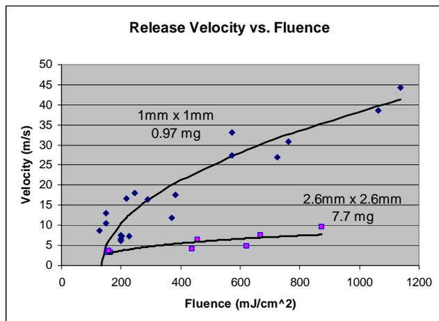
Fig. 4 Plot of velocity vs. fluence for two different sizes of bare dies.
