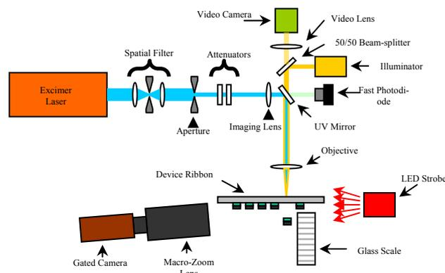
Fig. 1 Schematic of die transfer imaging apparatus.
