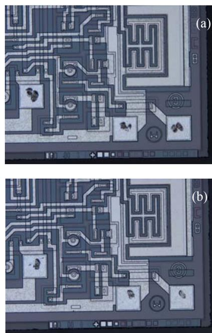
Fig. 5 a) LM555 bare die un-transferred. b) LM555 bare die after transfer.
