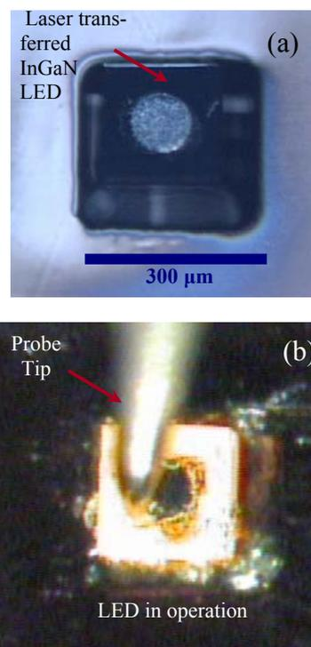
Fig. 6 a) Micrograph of laser transferred InGaN LED inside a receiving pocket. b) When powered, transferred LED emits light.
