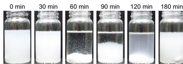
**Fig. 6** Temporal change of CaO colloid appearance in ethanol during LAL. The laser fluence was  $1.0 \text{ J/cm}^2$ . These pictures were taken while stopping stirring. While stirring, the gel-like structures observed in the 60 and 90 min samples were floating throughout the solution.
