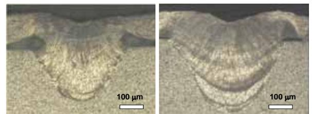
a) short tailing of laser pulse b) high laser peak power and long tailing of laser pulse
