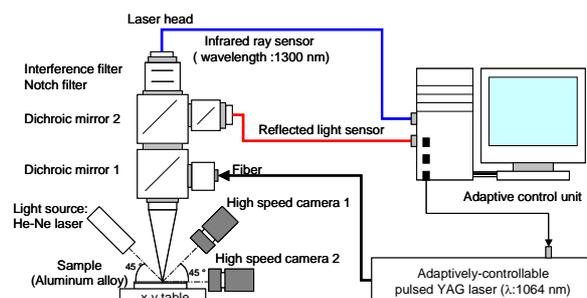
**Fig. 1** Schematic drawing of experimental set-up of in-process monitoring and adaptive control.
