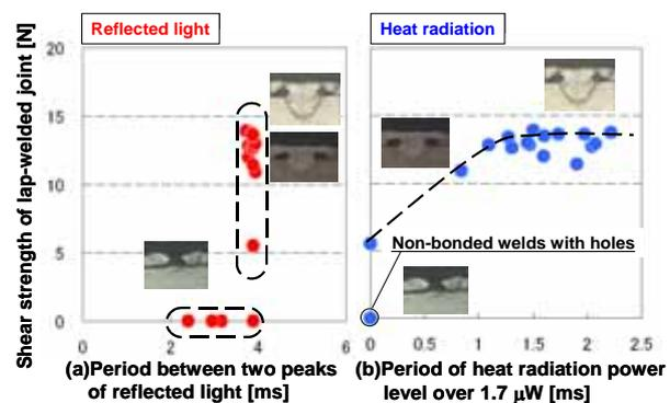
Fig. 6 Relationship of between monitoring signals to shear strength of lap-welded joint.
