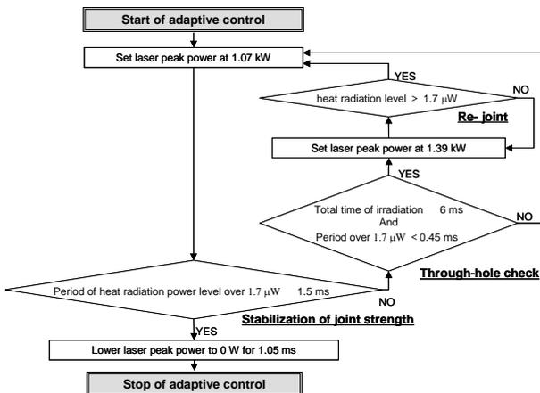
**Fig. 7** Flow chart of adaptive control based upon intensity level and period of heat radiation.
