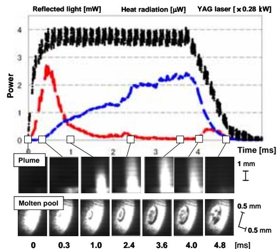
**Fig. 4** Monitoring results of laser micro-spot lap welding of A3003 sheets, showing high-speed observation images, pulse shape, reflected light and heat radiation signals.
