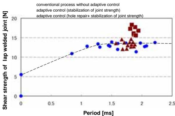
Fig. 10 Relationship between period of heat radiation power level over 1.7  $\mu$ W and shear strength of lap-welded joint made under adaptive control for hole repair in addition to data under conventional control.
