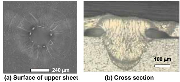
**Fig. 8** Surface and cross section of laser micro-spot weld produced in A3003 alloy under the adaptive control for the through-hole repair in the upper sheet.
