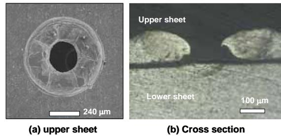
**Fig. 3** Top surface of upper sheet and cross section of a non-bonded A3003 weld with a hole.
