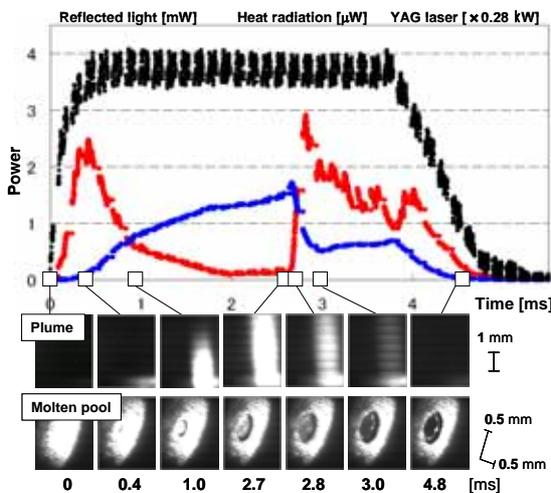
Fig. 5 Monitoring results of non-bonded welds with holes, showing high-speed observation images, pulse shape, reflected light and heat radiation signals.
