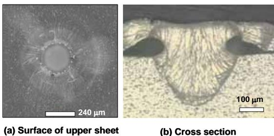
**Fig. 2** Surface and cross section of a laser micro-spot weld in A3003 alloy.
