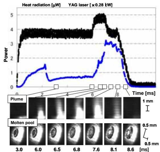
**Fig. 9** Monitoring results of the adaptive control, showing high-speed observation images, pulse shape and heat radiation signals.
