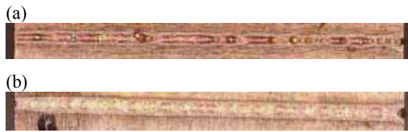
Fig.10 Optical images of bead on test with pure copper. (a) Conventional focused beam (b) with beam mode controlled technology
