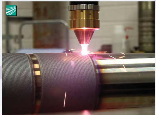
Laser cladding process using the COAXpowerline coaxial nozzle
